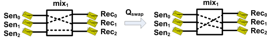
Figure 5: Q_{\text{swap}} transition operation on the second and third links of a mix
